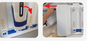
Before cleaning each Charging bay, Inspect the unit for damage. Paying special attention to highlighted areas in the diagram, ensure the gold contact pins are all fully extended and clean.
